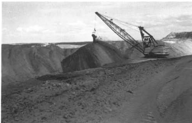
Figure 2. Dragline used to move overburden from above the coal seam to a mined-out portion of the operation. The bucket of the machine is large enough to carry two pickup trucks.
