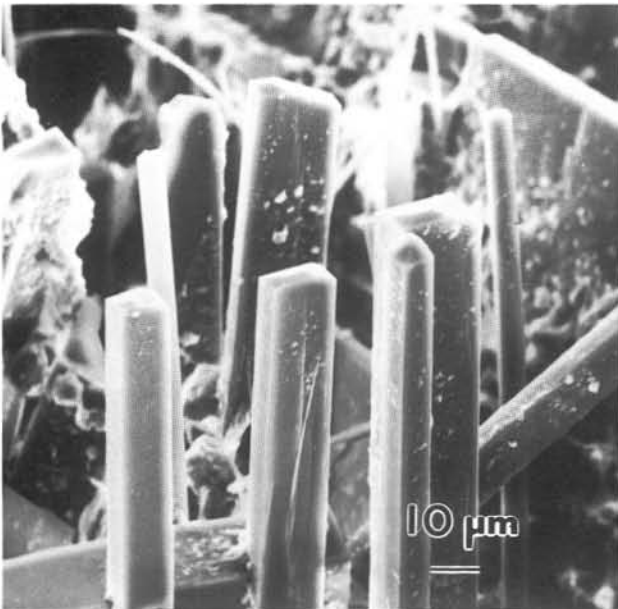
Figure 11. Scanning electron micrograph showing tabular thomsonite and later acicular scolecite crystals that coat fractures at 767-m depth.
