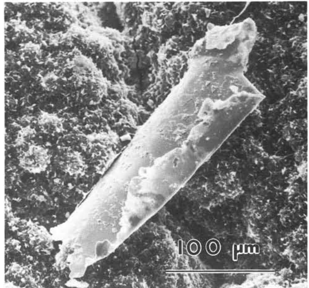
Figure 16. Scanning electron micrograph showing a deposit in an open space from 1,015-m depth consisting of native copper, later botryoidal clusters of \beta -cristobalite crystals, and still later smectite (fuzzy coating on \beta -cristobalite).
