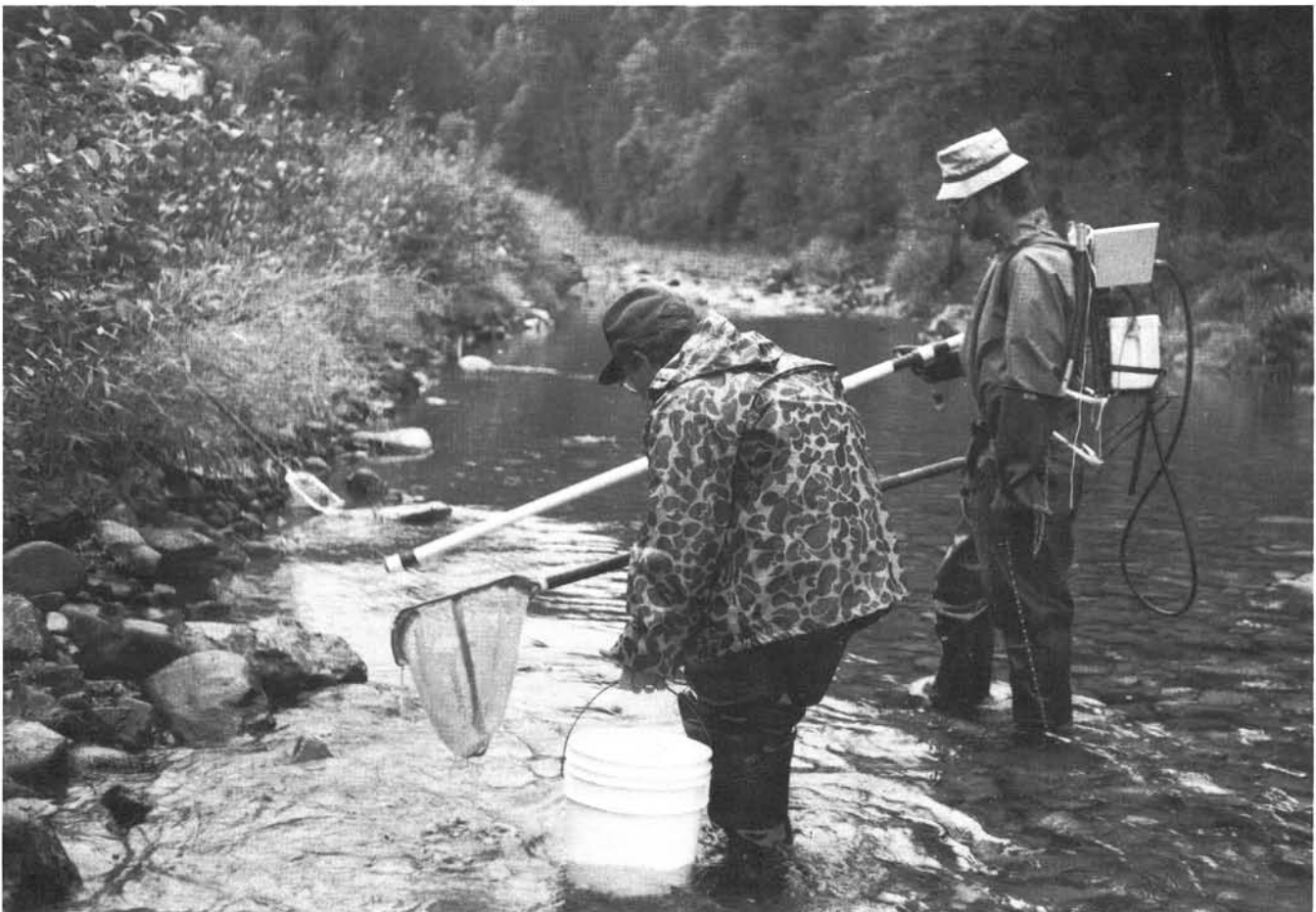
Figure 2. The electrofisher in the background stuns the fish so the netter can catch them.
